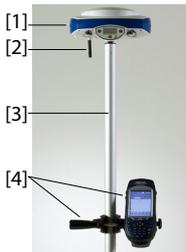
As a standard feature, the ProMark 500 incorporates a built-in GSM module, which means you only have to connect the GSM antenna if you have paid for activation of the hardware. Mount the different items as shown on the picture, including the ProMark 500 [1], the GSM antenna [2], the range pole [3] and the field terminal with its mounting bracket [4].
